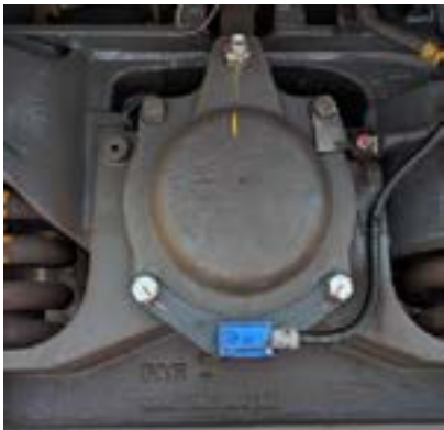
Figure 10: Axlebox sensor installed on C374
