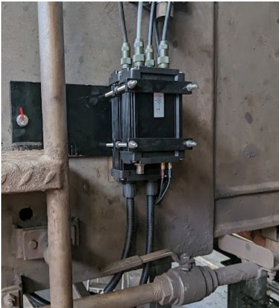
Figure 5: (Left) Vehicle body logger unit (Right) System mounted on under carriage of C374
